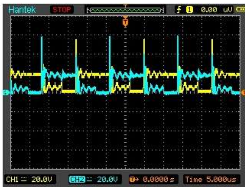
Fig.5. MOSFETs Drain Signals, for output current 2A and 12A.
